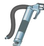
These should be checked periodically and replaced if found to be fraying, cut or damaged in any other way.
