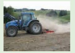
GMT300 fitted with Rotary Mulcher kit makes quick work of maize stubble
